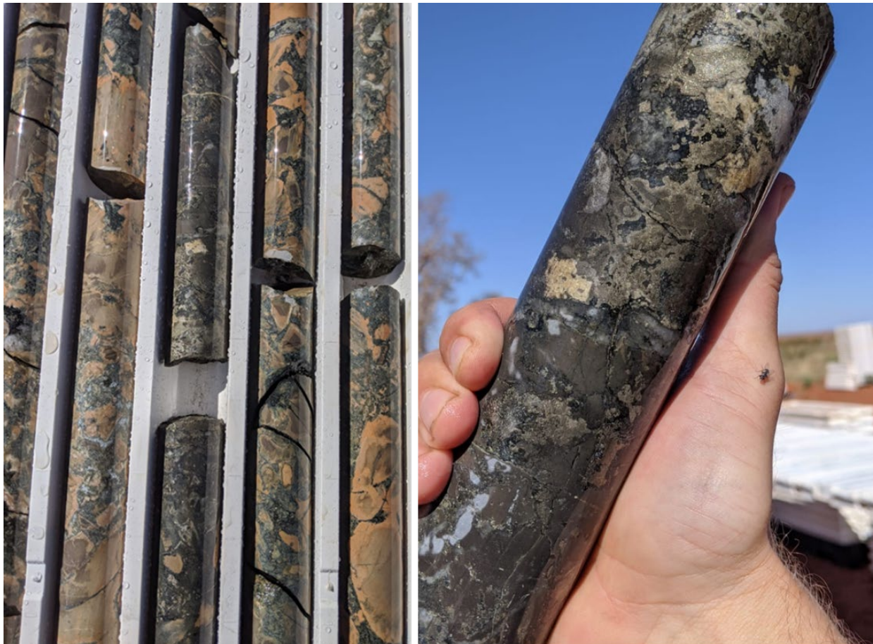
Photo 1: Drill core from ETG203 showing brecciated, silicified, hematite altered rock with pyrite and pyrrhotite, and amorphous quartz veining. Left (~185-190m) Brecciated and altered sediments containing disseminated and blebby sulphides. Right (~187m) Coarse euhedral pyrite and fine pyrite alteration within silicified and brecciated sediment 8
