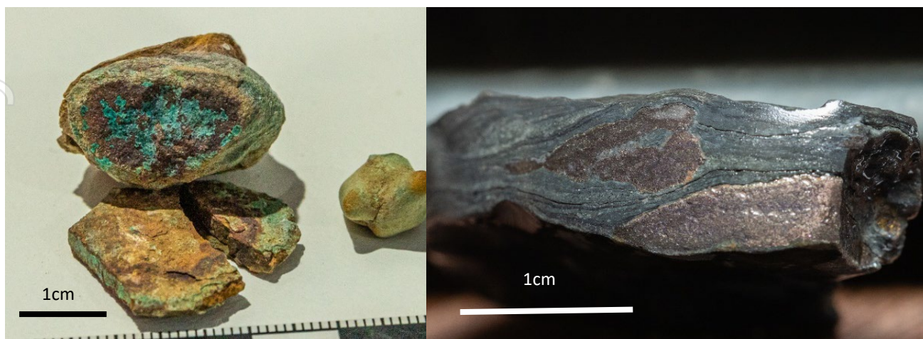
Photo 3 (left) – weathered copper rich nodules collected from surface at Area 1 (refer Figure 6) - containing malachite (interpreted after bornite-chalcopyrite), visual estimate 10% malachite in 2.5cm diameter nodule Photo 4 (right) – primary copper rich nodule from historical drillhole (Mt Skinner DDH3 203.3m) located adjacent to Area 4 (refer Figure 6) containing bornite-chalcopyrite, visual estimate 30% bornite-chalcopyrite over ~1cm width. 10
