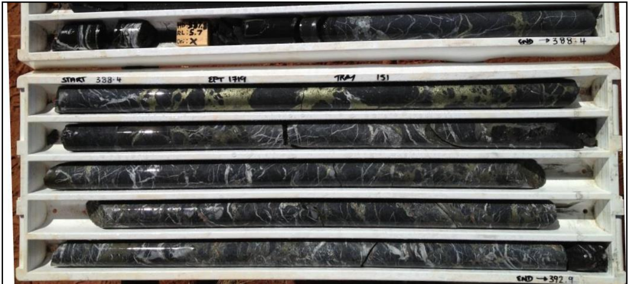
Photo 1 - EPT1719 – ~388m to 392.9m – Veined and brecciated carbonate with local massive copper sulphide breccia cement
