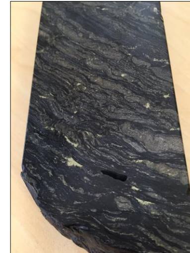
Disseminated chalcopyrite in carbonaceous shale EPT 2282 (~259.5m downhole (1.0%Cu)
