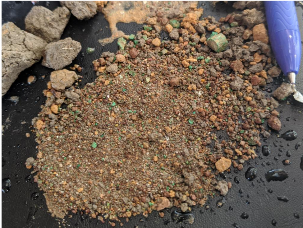
Photo 3 – Copper Carbonate (Malachite) mineralisation at Jessica: 0-3m from RN28419 – chemical assay 1.5% Cu
