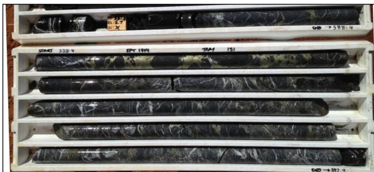
Photo 2: EPT1719 - ~387.6m to 392.9m (5.3m @ 2.5% Cu) – Veined and brecciated carbonate with local massive copper sulphide breccia cement 14
