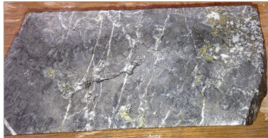
EPT1716 – ~120m - Carbonate with dolomite blebs/veins containing chalcopyrite (HQ core width 60mm)
