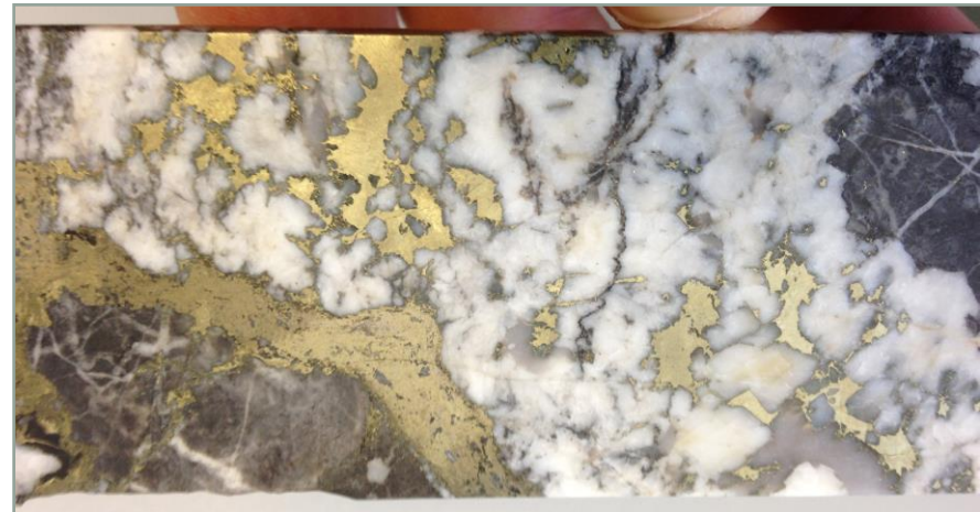
EPT1718 – ~285m - Carbonate/quartz vein containing chalcopyrite and pyrite (NQ core width 45mm)
