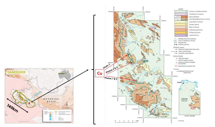
Figure 1 – Geology plan showing mapped cupriferous outcrop at Sandover (NTGS Kruse et al, 2013)
