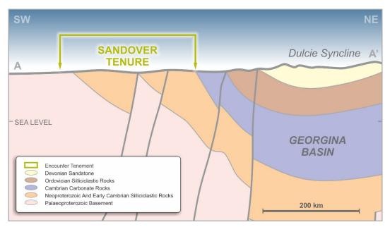
Figure 3 - Sandover Schematic Cross Section A-A'
