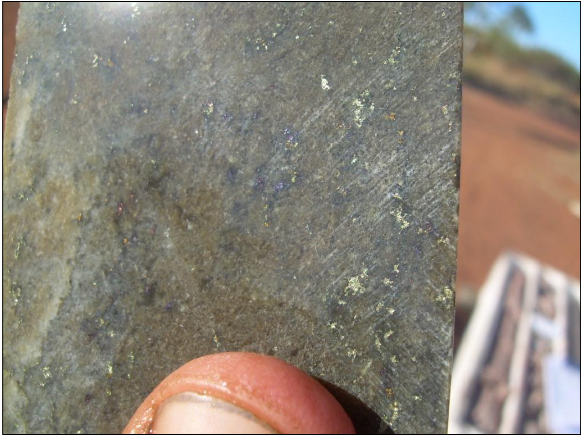
Photo 1: EPT801 (T4) 194.4m. Disseminated chalcopyrite and bornite in altered metamorphics
