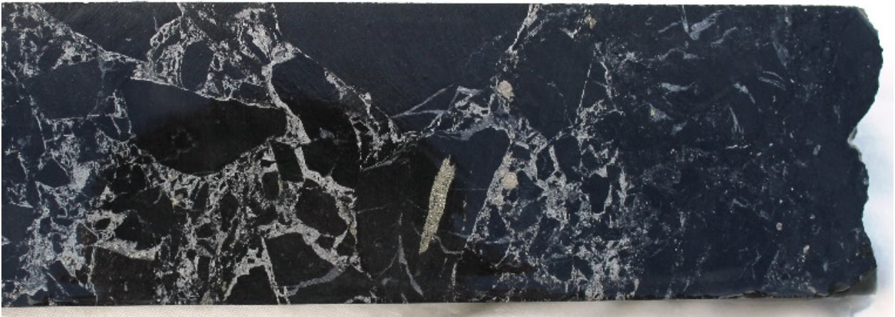
Photo 2: Millennium prospect – EPT2198 (~295m) Sphalerite (light brown) and minor pyrite in brecciated shale core sample width approx. 50mm
