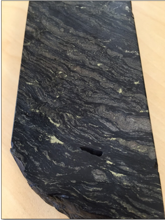
Photo 1: Disseminated chalcopyrite in carbonaceous shale EPT 2282 ~259.2m downhole (1.0%Cu) core width ~60mm
