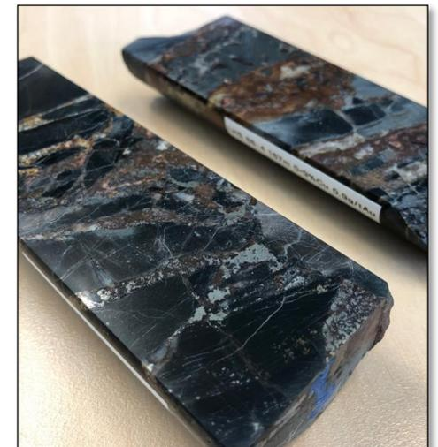
LHS 88-4 (Newmont, 1980s) ~155m and 167m. Veined and brecciated siltstone with pyrite and iron carbonate alteration.
