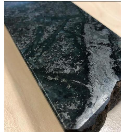
LSPC-3 (Newmont, 1980s) ~44m. Veins and disseminations of pyrrhotite and minor chalcopryite within an altered calcareous sediment.
