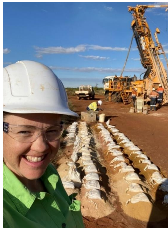
Photo 1: Encounter Exploration Manager Sarah James with RC pre-collar spoils from drillhole EAL008
